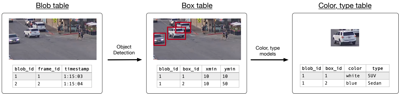
Figure 2: Example of a data model for a traffic camera dataset. An object detection model takes a frame (associated with a blob id) and produces a list of object types and positions. Given the list of cars, a separate ML model produces the car type (e.g., sedan vs SUV) and color.
